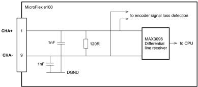
Figure 12 - Encoder channel input circuit - Channel A shown
